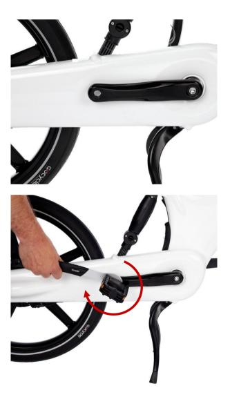
1.1. Undo and remove the original pedal as demonstrated.
